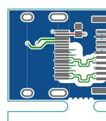
HDMI firewall dongle, top, scale = 1:1.000
