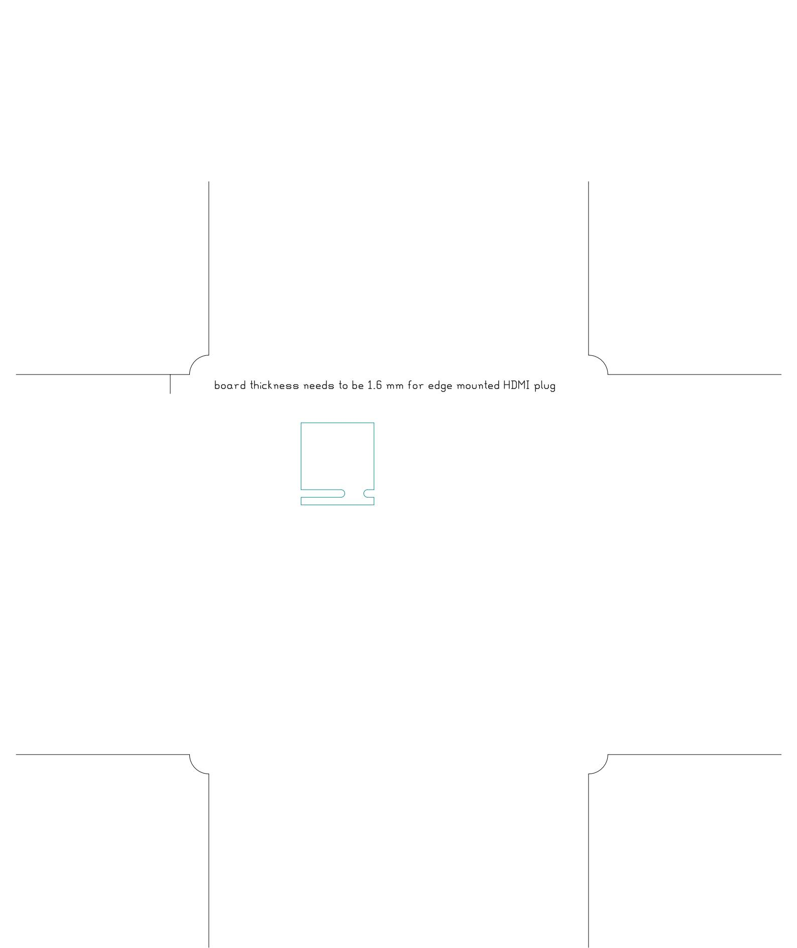
board thickness needs to be 1.6 mm for edge mounted HDMI plug
