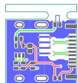
HDMI firewall dongle, bottom (mirrored), scale = 1:1.000
