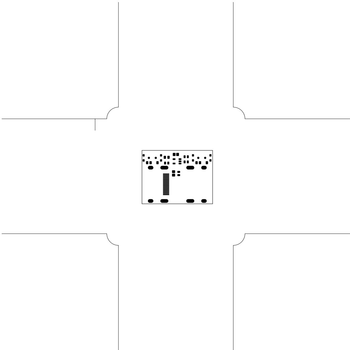
HDMI firewall, topmask, scale = 1:1.000
